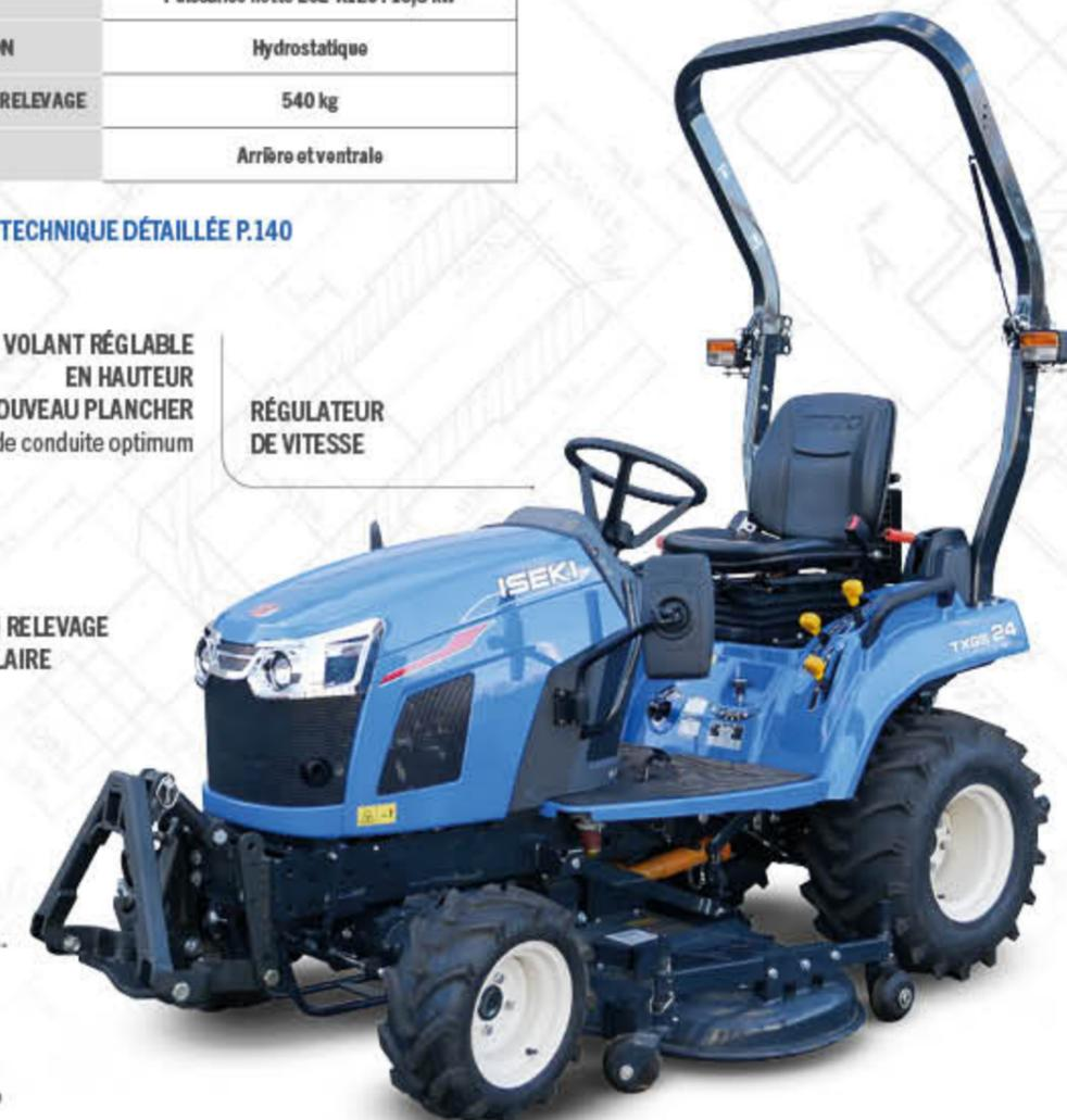
ARCEAU DE SÉCURITÉ ROPS REPLIABLE
